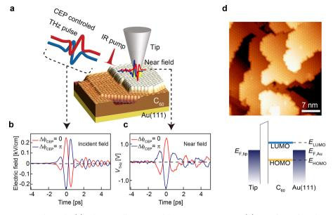
**Figure 1.** Measurement system and sample. (a) Schematic illustration of the measurement setup. (b) Waveform of incident electric field for  $\Delta \Phi_{CEP} = 0$  and  $\pi$ . (c) Waveform of near-field electric field for  $\Delta \Phi_{CEP} = 0$  and  $\pi$ . (d) STM image of the sample. (e) Band diagram of the STM tunnel junction at equilibrium ( $E_{LUMO} - E_{F,Au} = 0.9$  eV,  $E_{F,Au} - E_{HOMO} = 2.2$  eV).
